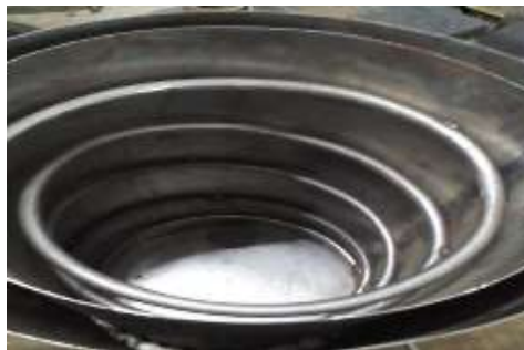
Fig. 5 Welding of Steel Pipe to the Drum
